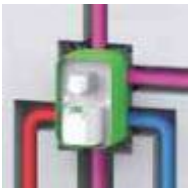
2 (1). According to the site condition and the installation size requirement to set up the pipe line (2). Connect the plastic box to the pipe, put the plastic box on the hole, then adjusted the levels (the bubble on the middle of the leveller). (3). Make the positioning holes.
